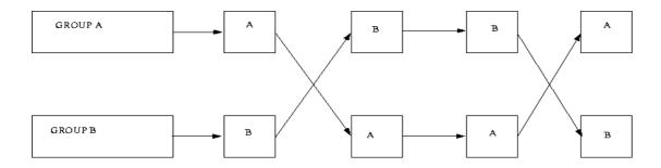
A product is alternating between students during the fabrication process. When produced by student A at a certain stage then student B will carry out the quality control of the part. Student B will then use the part from A in his own production and then transfer it back to A for the following quality control.
