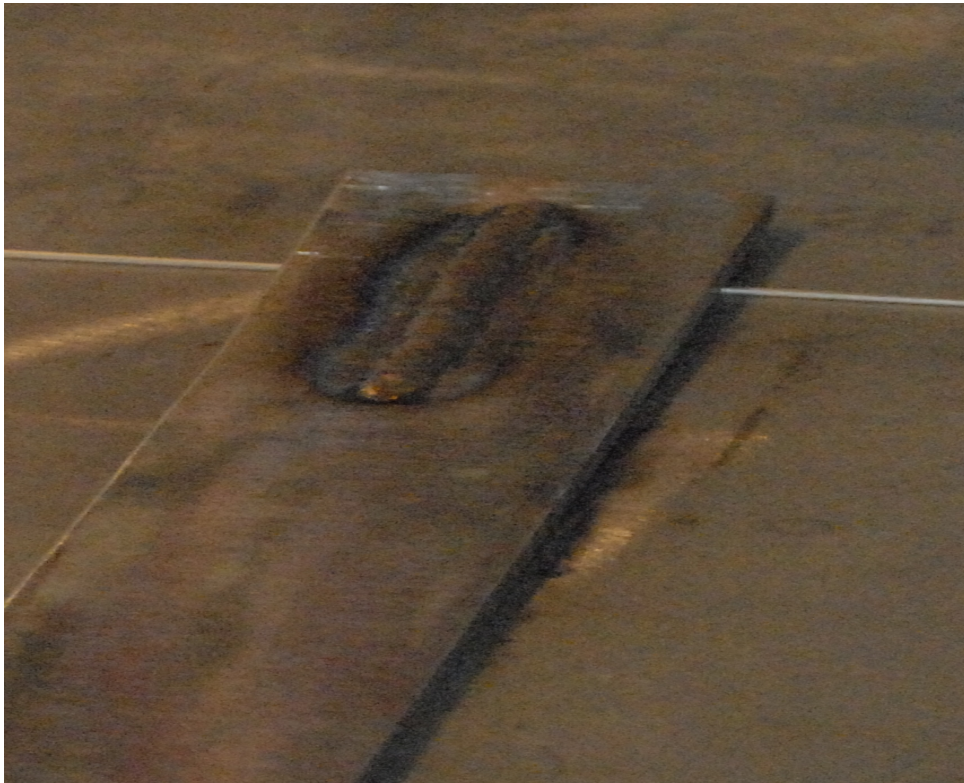
Fig 13. A photo of a clad weld as described above. A 3 mm rod has been rolled under the plate which has bent upwards.
