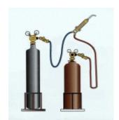
oxygen cylinders have a right-hand and acetylene have a left-hand thread. All cylinders are opened by turning the key or knob anticlockwise and closed by turning them clockwise.
